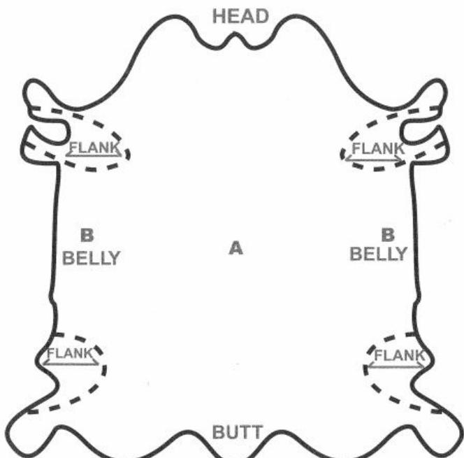
SECTION A should be used in cutting seat tops, inside back, cushion bands and other sections that will see the most strain and use. This is the prime portion of the hide.
